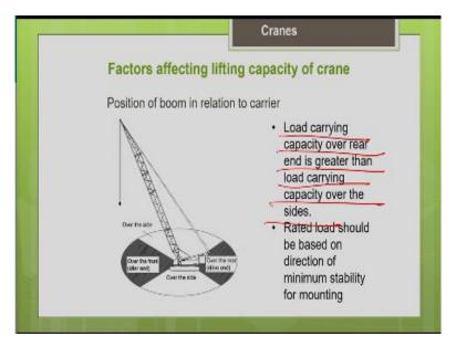
Another important thing is, as the boom of the crane rotates so you can see that the lifting capacity possible varies. You can divide it into four quadrants. You can see in this picture. When the boom is in the front end or the boom can be in the rear end or boom can be to the right side or left side so, boom can be in the side of the carrier or boom can be in the front end with respect to the carrier or boom can be the rear end with respect to the carrier.
