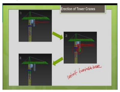
Once this is done, then you can do the self-erection of the tower crane. So, how to do that? First, what you do is, you have to introduce a new section to increase the height of the tower crane with the help of trolling action. You know the trolling rate. There is a trolley here in the main jib. By the trolling action so, you can bring the, you see, here you can see, this is a new section.
