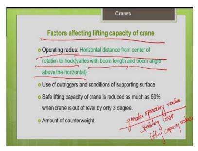
So far, we have discussed about the different types of tower cranes on the basis of method of slewing, top slewing, bottom slewing and on the basis of the type of boom, horizontal boom, luffing boom and articulated jib and special tower cranes like climbing tower cranes particularly for very tall structures. All these things are discussed. Now, let us move on to the next topic, what are the factors what are the affects the lifting capacity.
