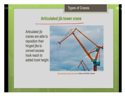
There is another type of jib apart from the horizontal boom, luffing boom. You also have this articulated jib tower crane. You can see the picture. See, these articulated jib cranes are able to reposition their hinged jibs to convert the excess hook ridge to added hook height that means so, you can reposition the jib in such a way that. So, whenever you do not need excess horizontal reach, you can convert the horizontal reach into vertical height.
