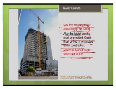
So, another important thing, you need to know that is the maximum free standing tower crane height permissible is 60 to 120 meter. So, beyond 120 meters, the tower crane should take the help from the structure. You should properly brace it to the nearby structure to transfer the overturning movement to the structure from the stability point of view. So, after 120 meters, definitely should provide the lateral bracing. The crane must be tied to the structure and the construction.
