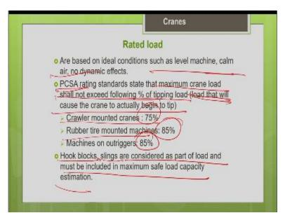
So, the rated load as I told you, the crane rating, the load rating is done based on ideal conditions assuming that the machine is level; the surface is level; the air is calm; the wind speed is not high; there are no dynamic effects. Based on this assumption only, rating is given. If your conditions are going to be different, so, the lifting capacity must be reduced accordingly. So, as I told you in the earlier lecture, there is an organization called PCSA Power Crane Shovel Association.
